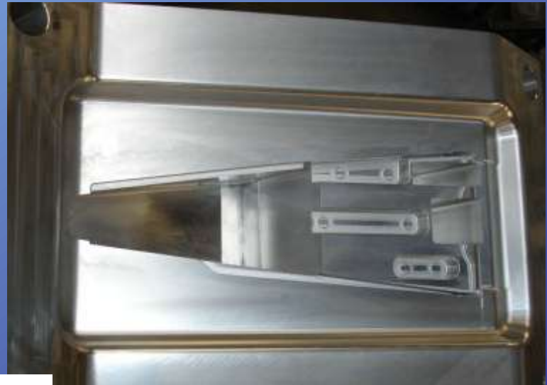
Motorbike Back wheel cover in plastic made by Ci-ESSE mould
