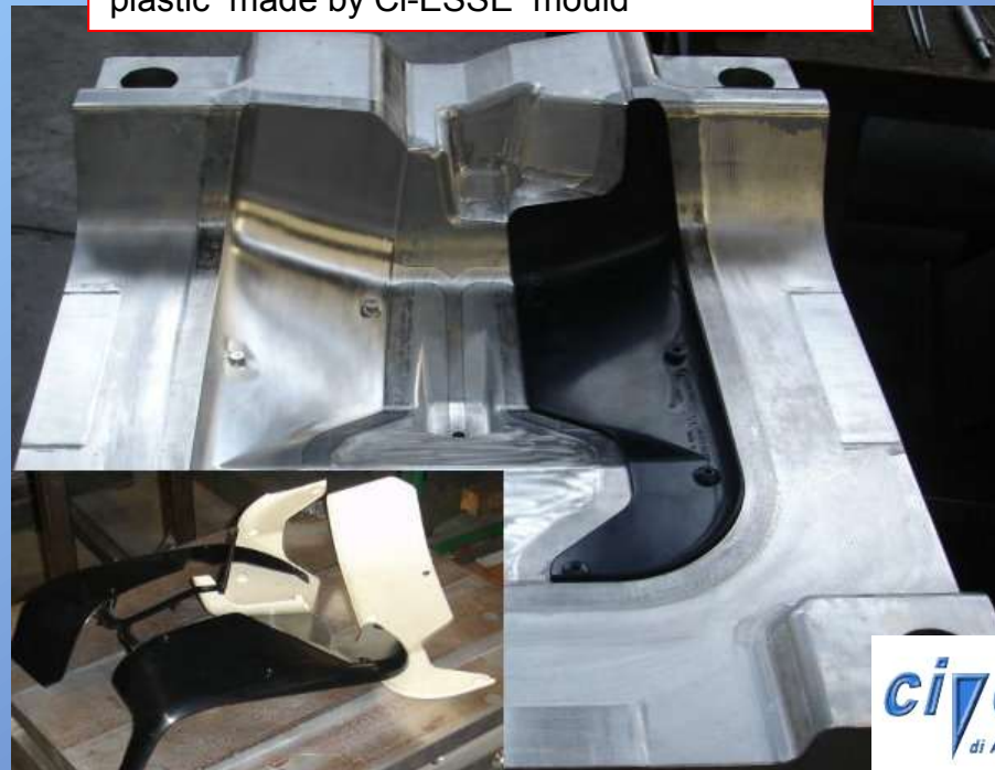
Motorbike Lower LH & RH leg protection in plastic made by Ci-ESSE mould
