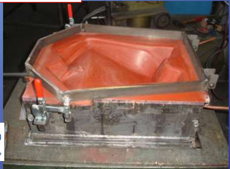
Motorbike Back seat PU+ Vacuum forming PVC made by Ci-ESSE resin mould
