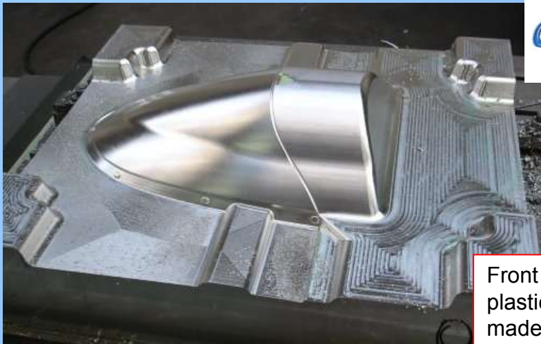
Motorbike Lower LH & RH leg protection in plastic made by Ci-ESSE mould
