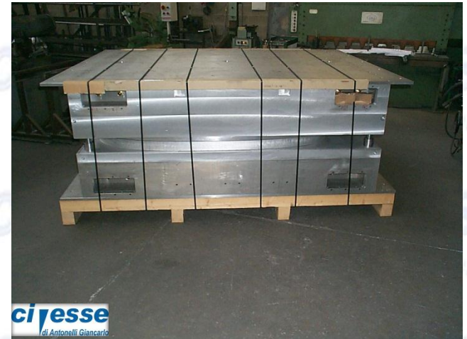
A female-male vacuum formed tool
