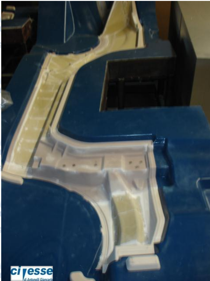
Proto-tools ureol + resin + alu inserts for p-DCPD tech
