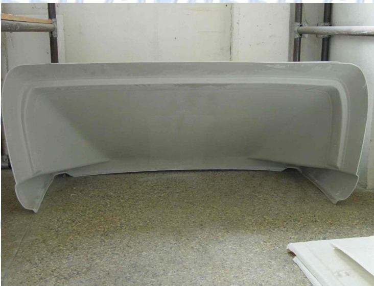
Large roof spoiler and structure in RTM light By Ci-ESSE epoxide resin molds
